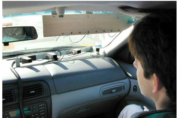
Figure 1: Eight microphones on the sun visor, four cameras on the dashboard.
